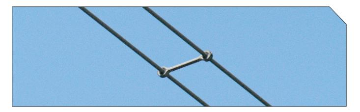
PLP's Twinlok spacer is designed to meet Australian standards combining strength and performance, while still maintaining a lightweight design. The semi-conductive cushion inserts protect the outer stranding of the conductor, whilst the strengthened aluminium frame is designed to protect against conductor clashing without deformation.
